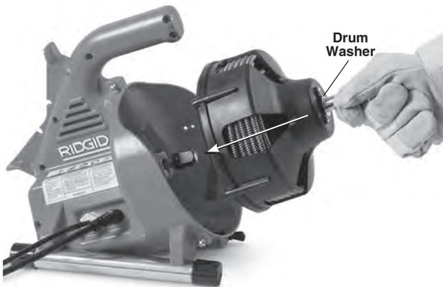
Figure 16 – Inserting Drum Into Machine
